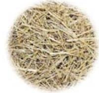
The extended-term erosion control blanket shall be a machine-produced blanket of 70% agricultural straw and 30% coconut fiber matrix with a functional longevity of up to 24 months. (NOTE: functional longevity may vary depending upon climatic conditions, soil, geographic location, and elevation).
