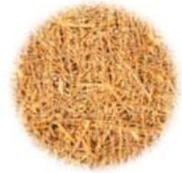
The short-term double net erosion control blanket shall be a machine-produced 100% biodegradable blanket with a 100% agricultural straw matrix with a functional longevity of up to 12 months (NOTE: functional longevity may vary depending upon climatic conditions, soil, geographic location, and elevation).
