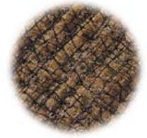
The composite turf reinforcement mat (C-TRM) shall be a machine-produced mat of 100% coconut fiber matrix incorporated into a permanent three-dimensional turf reinforcement matting.
